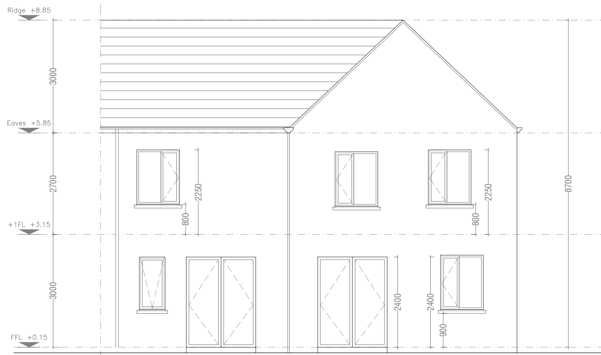
House Type P1 Terraced Rear Elevation
